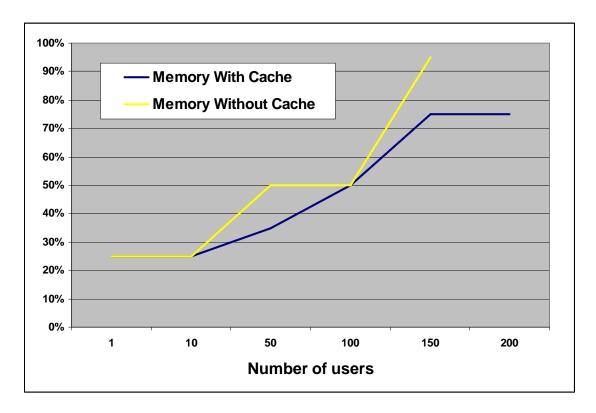
Figure 4: Memory used on Zend Engine Server.
