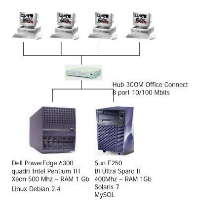
Figure 5: Platform used in performance measurements
